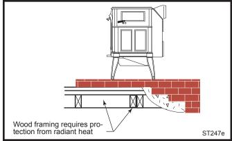
**Fig. 11** Combustible supporting timbers may lie beneath fireplace hearths, reqireing additional floor protection.
